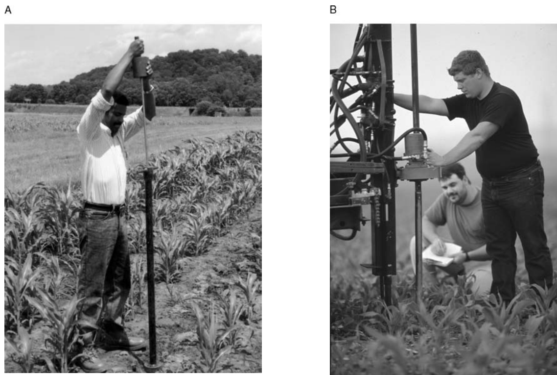
FIGURE 3.24 A. Uhland drop hammer bulk density sampler. B. Hydraulic soil coring device.
