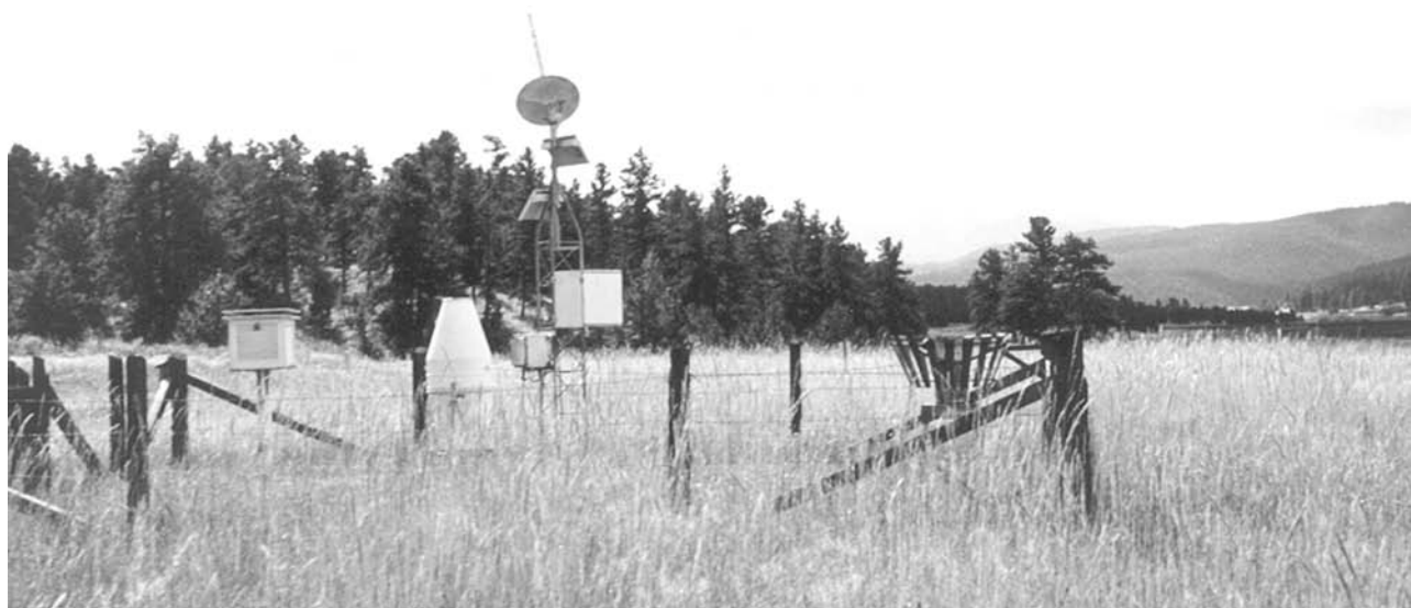
FIGURE 2.12 Weather station at the Manitou Experimental Forest near Denver, CO. The instrumentation from left to right is as follows: screened box with thermometers; strip-chart recording rain gage; tower with tipping bucket rain gage; electronic temperature sensor solar panel to recharge system batteries; antenna to relay recordings to central site via satellite; d box with data logger instrumentation; and 8-in. standard rain gage with windshields. In the background is Pike's Peak. (Photography by W. Elliot.)
