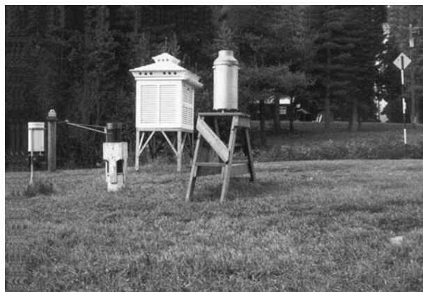
FIGURE 2.10 Weather station at the Priest River Experimental Forest in northern Idaho. The instrumentation from left to right is as follows: tipping bucket rain gage; sunshine recorder; solar radiation pyranometer; standard 8-in. rain gage; screened box containing thermometers for maximum, minimum, and wet-bulb temperatures; and strip-charge recording rain gage. The striped post with a diamond-shape sign in the background is one of the points on the snow survey course around this site. (Photography by W. Elliot.)
