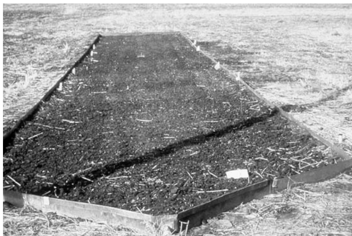
FIGURE 9.9 Fallow soil erosion plot located near Pullman, WA, with a standard length of 72.6 ft and a slope steepness of about 9%.
