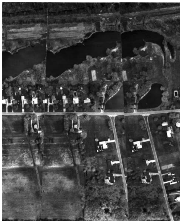
FIGURE 13.4 Lower altitude stereoscopic coverage (Ohio) acquired for engineering purposes, typical of the photographs available from state departments of transportation. Note the presence of two lakes, ditches, trees, and homes and how stereoscopic viewing supplies additional information about the area.
