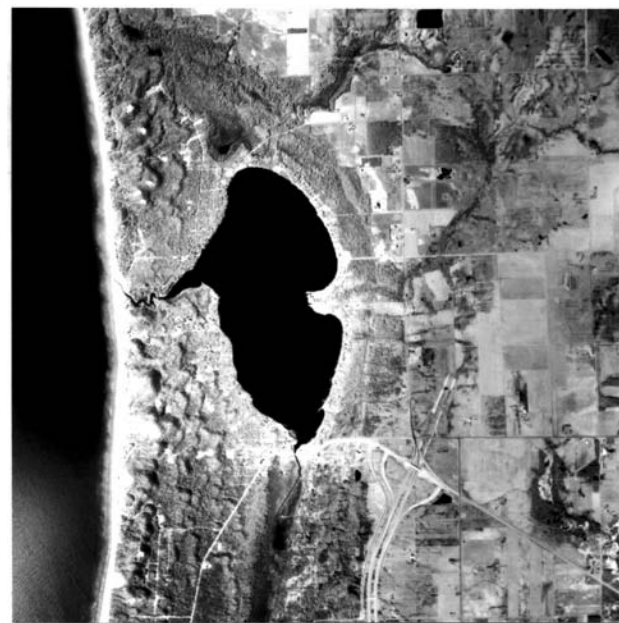
FIGURE 13.2 The difference in this image (April 18, 1981) of the same location in Figure 13.1 is because the film is black-and-white infrared. Note the lack of detail within the water due to the absorbance of infrared light at the surface and near surface of the water. The infrared film helps identify the location and surface area of water bodies.
