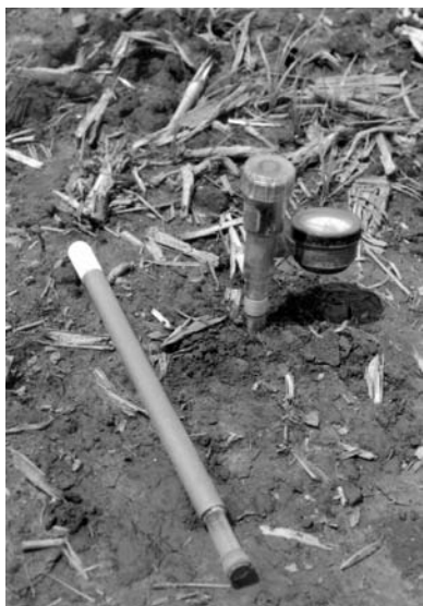
FIGURE 3.27 Tensiometer methods for measuring in situ soil suction.
