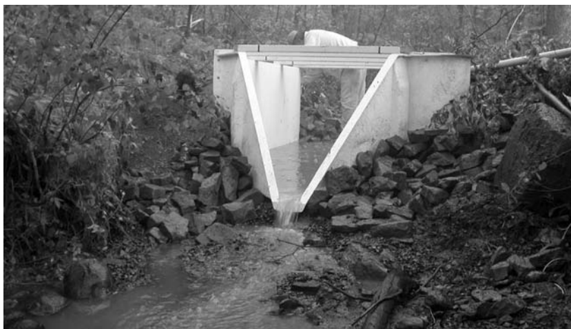
FIGURE 8.3 Flume in a stream. (Courtesy Kevin King.)
