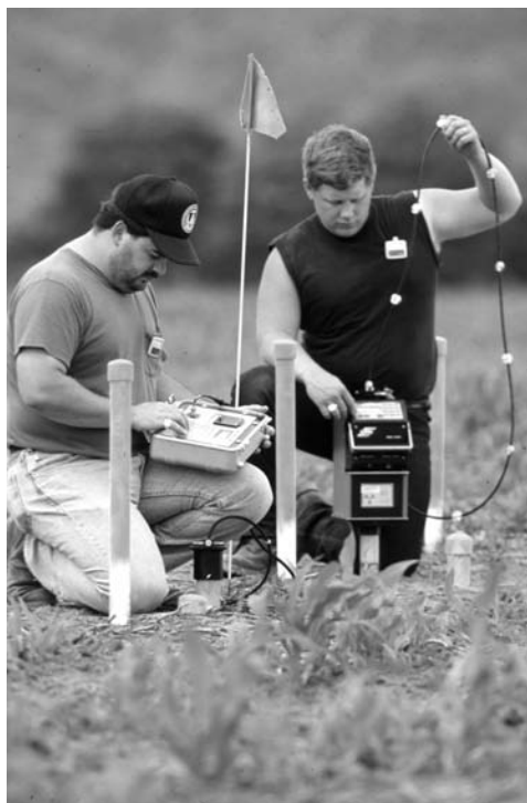
FIGURE 3.25 Indirect method for measuring bulk density or soil moisture content of a soil.
